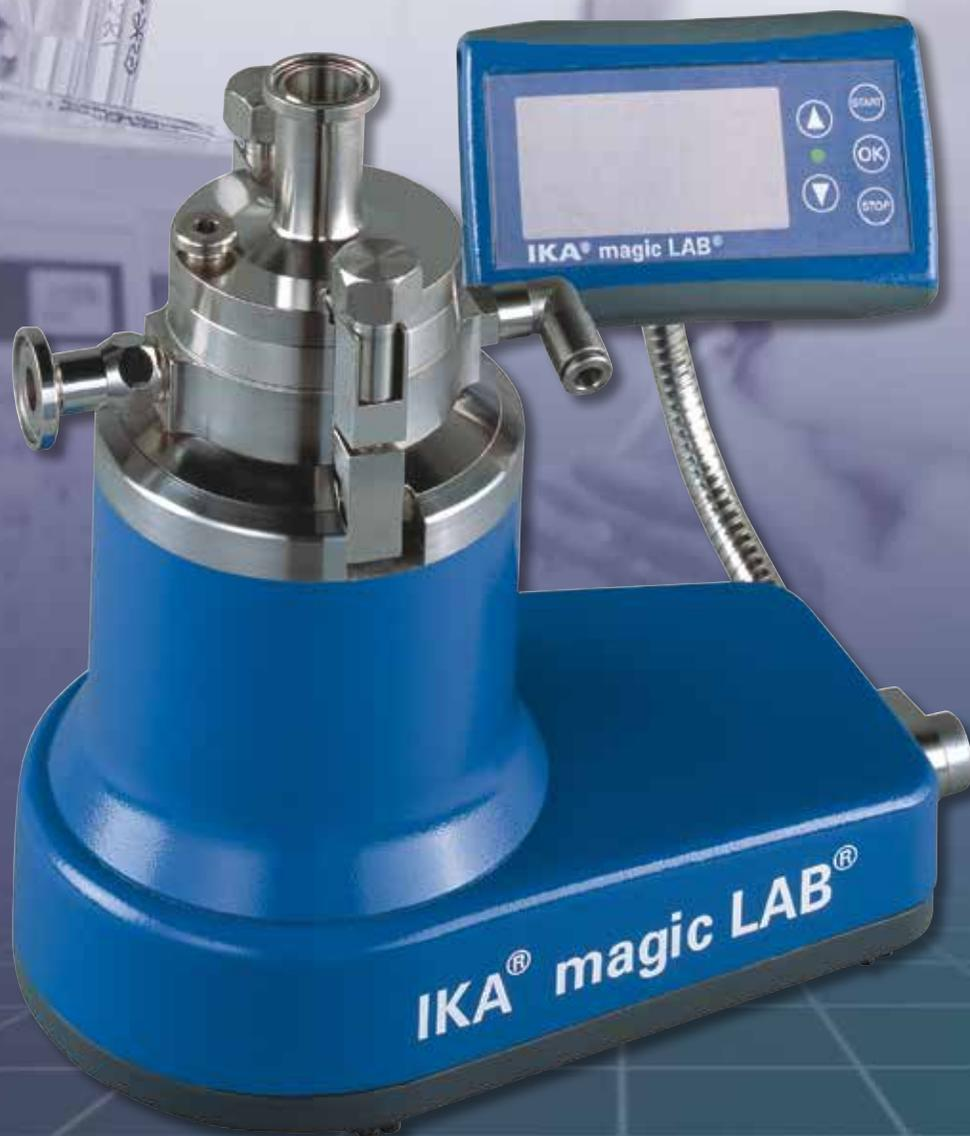
Wet Grinding – Fine Grinding – Emulsifying – Dispersing/Mixing – Powder/Granule Incorporation
